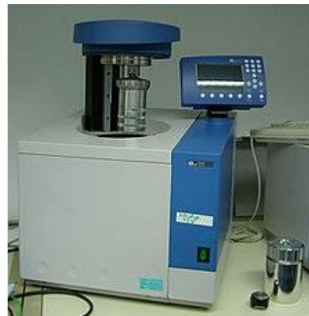
Figure 6. Bomb Calorimeter for CV determination
