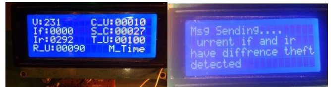
Figure 12. Experimental results of shorting phase or neutral line.
