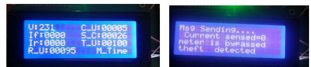
Figure 13. Experimental results of whole meter bypassing.
