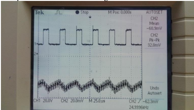
Figure 5. PWM and Current results from the hardware
