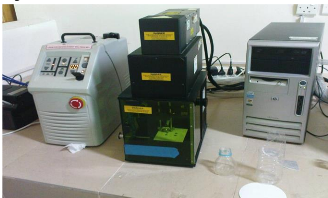
Figure 2. LIBS apparatus setup with PET plastic bottle sample
