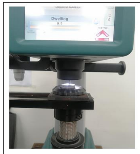
Figure 2. Sample is placed on specimen holder and indenter apply load on sample of 1 kgf for 10 second
