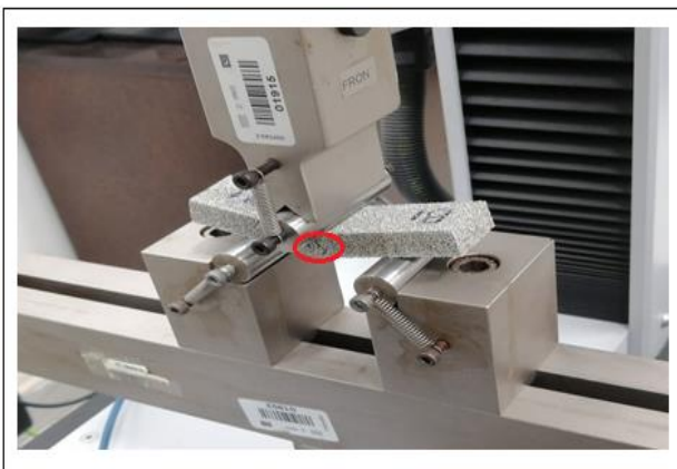
Figure 1. Three point bending test machine apply load with 1 mm/min on sample until fracture
