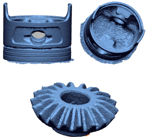
Figure 6. Resulted Solid Mesh Model using Photogrammetry
