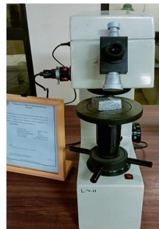
Figure 10: Performing Vickers Hardness Test
