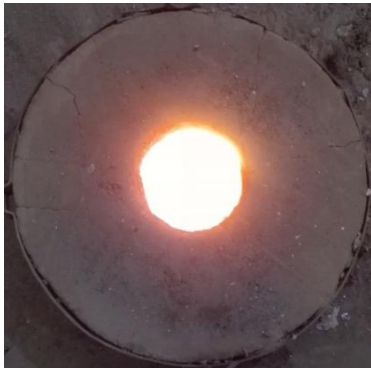
Figure 4: Pit Furnace for Alloy melting
