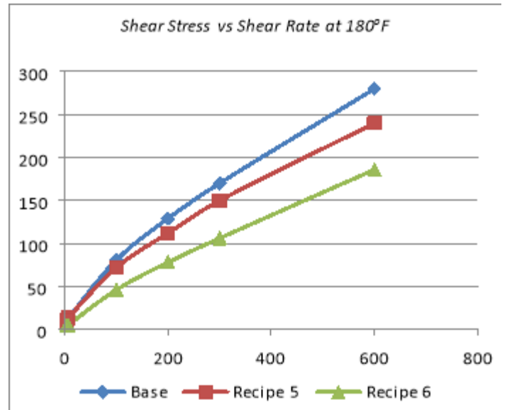
Figure 14 Graph of Shear stress against Shear rate for base case, recipe 5 & recipe 6 @ 180°F
