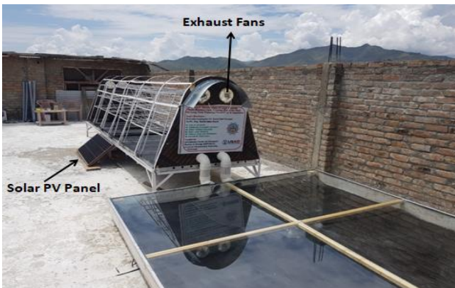
Figure 2: Solar PV system (Dryer installed in SWAT)
