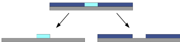
Fig. 9 Schematic mask and etch sequence. Mask patterning is done initially to open ARC, followed by a process of photoresist removal
