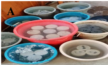
Figure 3. Different mix designs and making of final geopolymer concrete; A) Dry mixing of raw materials, B) Different mix designs, C) Mixing Chemicals, D) Paste prepared, E) Molding of concrete, F) Final Samples prepared.
