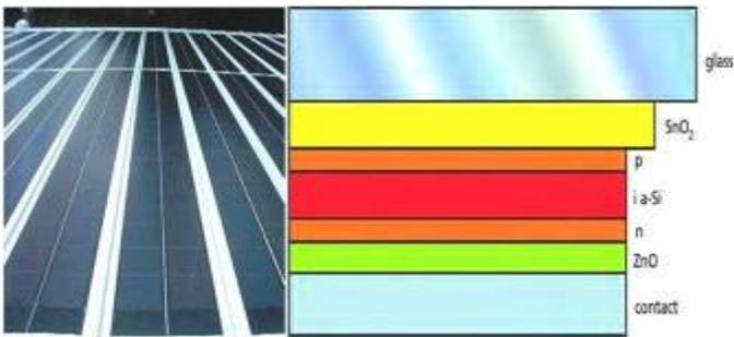
Figure 9. Amorphous modules and amorphous cell layered structure
