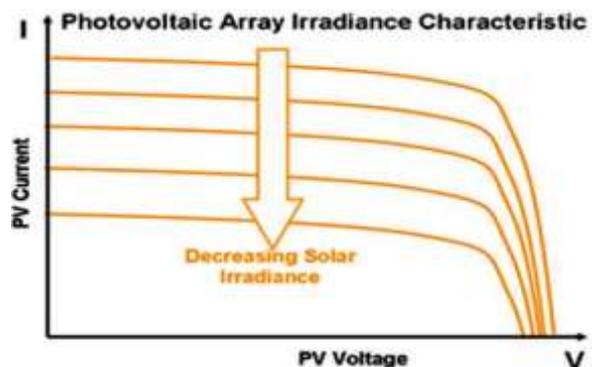
Figure 1. Effects of irradiance on current and voltage of PV module
