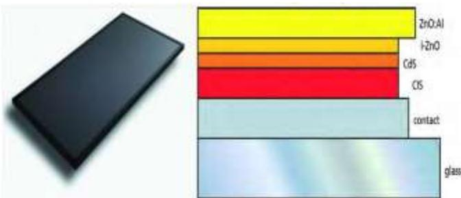
Figure 10. CIS module and CIS cell layered structure
