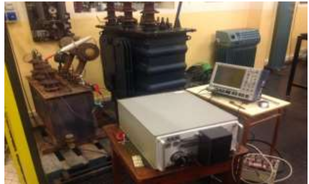
Fig1. Experimental setup for transformer testing
