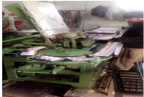
Figure 4. Installation of steel racks on Box Filling Machines
