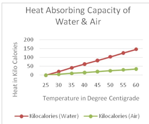
Figure 12. Heat Absorbing Capacity of Water & Air
