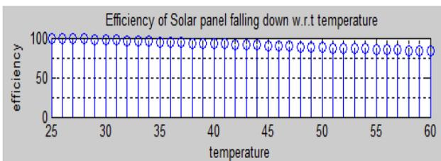
Figure 4. Efficiency vs Temperature in the absence of Water
