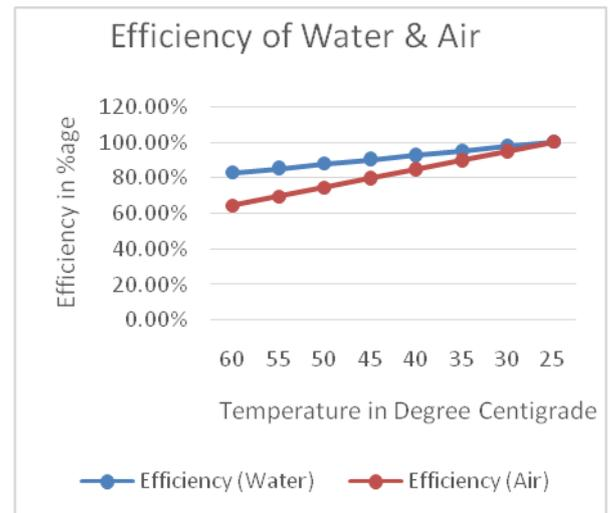
Figure 10. Efficiency of Water and Air
