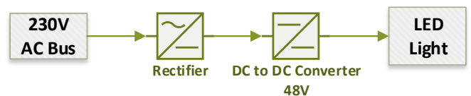
Figure 10. LED Light in AC nanogrid
