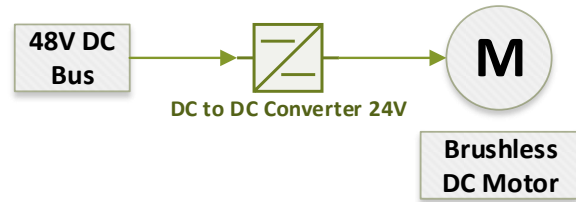
Figure 15. DC fan/refrigerator in DC nanogrid
