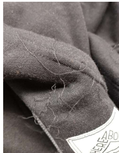
Figure 2. Uncut thread defect.
