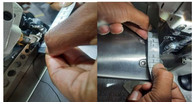
Figure 9. Thread cutter installed on Over-Lock machine.
