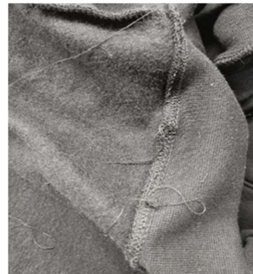
Figure 8. Uncut thread defect caused by Over-Lock Machine
