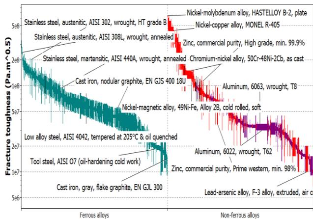
Figure; 4 Illustrate the fracture toughness (Pa.m<sup>0.5</sup>) against the metal alloys.
