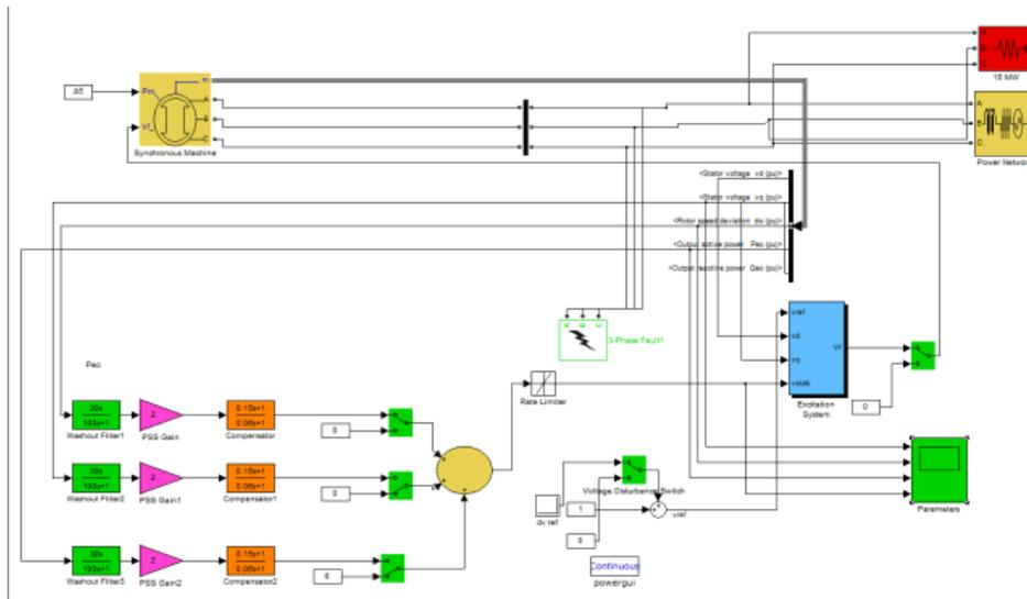
Figure: 5 Simulink Model with Power System Stabilizer
