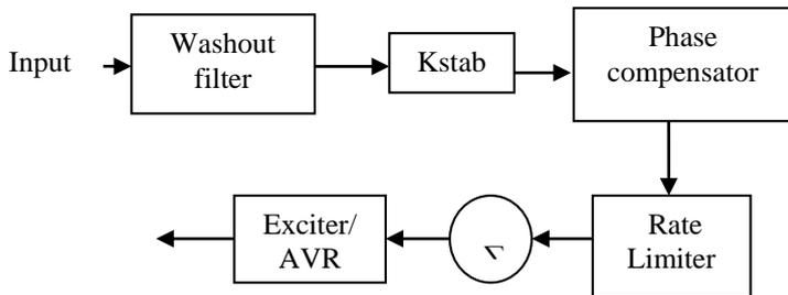
Figure 1: Block Diagram of PSS
