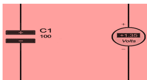
Figure 9 Battery cell in Proteus capacitor used
