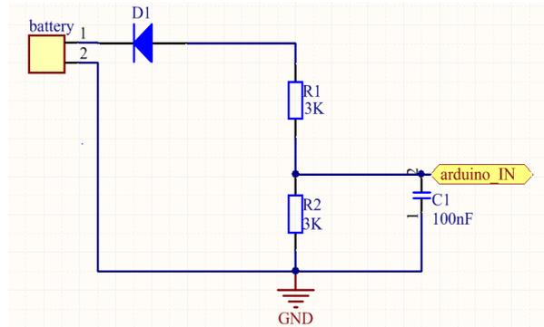
Figure 3: Circuit diagram for battery status
