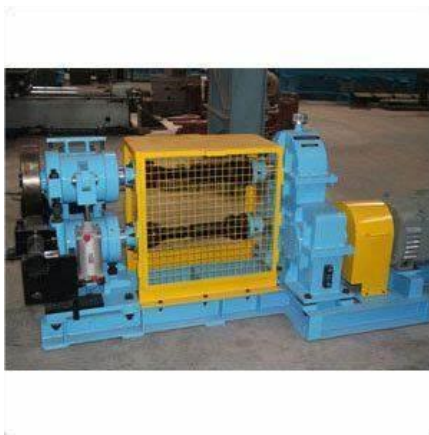
Figure 7. Pinch roller
