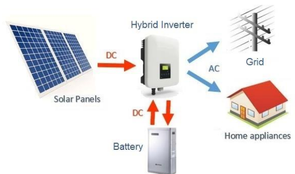
Figure 8. Hybrid Solar PV System
