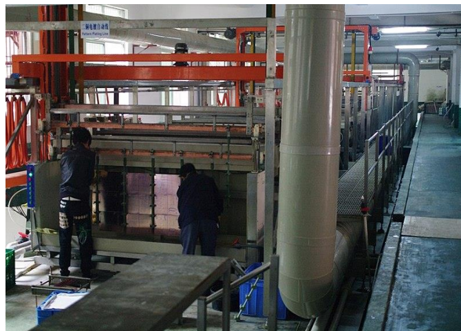
Figure 3: Process of Electroplating and its complex machinery (Source: Wikipedia contributors 2024)
