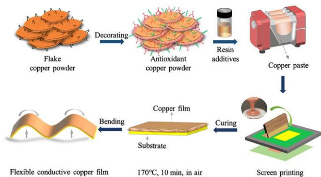
Figure 10: General scheme for fabricating antioxidant copper paste and screen-printing flexible electronics. (Source: Hong et al., 2022)
