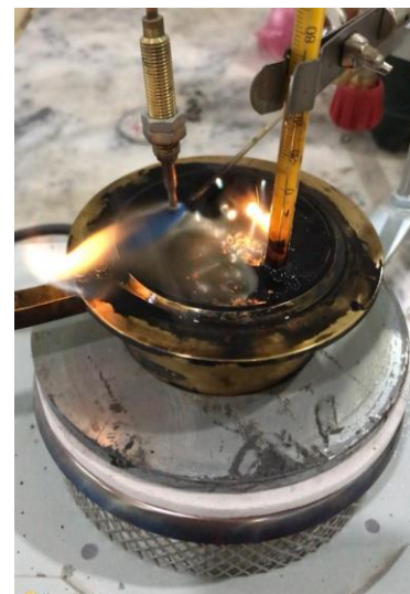
Figure 4. Flash & Fire Point test
