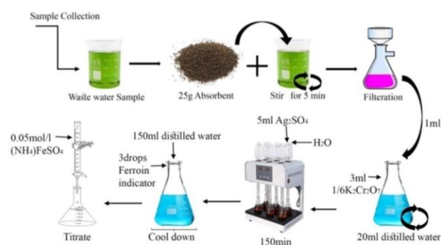
Figure 3. The flow chart for COD treatment and determination.
