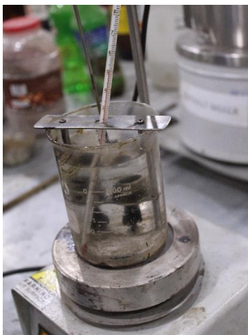
Figure 2. Softening Point test
