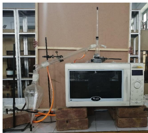
Figure 2: Microwave Assisted Distillation
